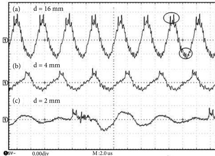
Figure 2. Oscillogram of the discharge current for corona (a), (b) and arc (c) at various distance  $d$  between the high voltage electrode and agar surface (a vertical division corresponds to 5 V; a horizontal division — 2  $\mu$ s; the curves show 30 ohm resistance drop; current spikes due to streamer-type discharge are marked by circles)
